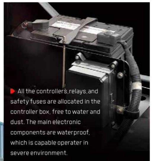
► All the controllers, relays, and safety fuses are allocated in the controller box, free to water and dust. The main electronic components are waterproof, which is capable of operating in severe environments.
